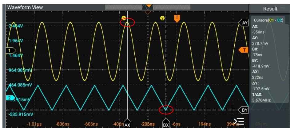
Figure 10.12 Track Measurement (before Horizontal Expansion)
