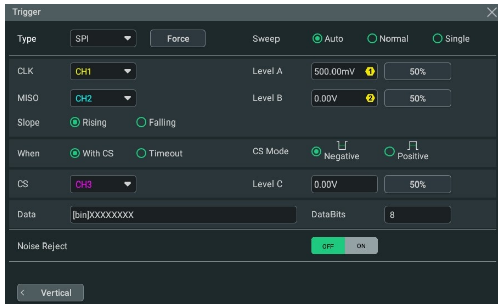
Figure 8.31 SPI Trigger Setting Menu
